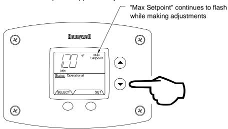
Step 4: Press "Set" button to confirm new "Max Setpoint" value and stop setting mode.
